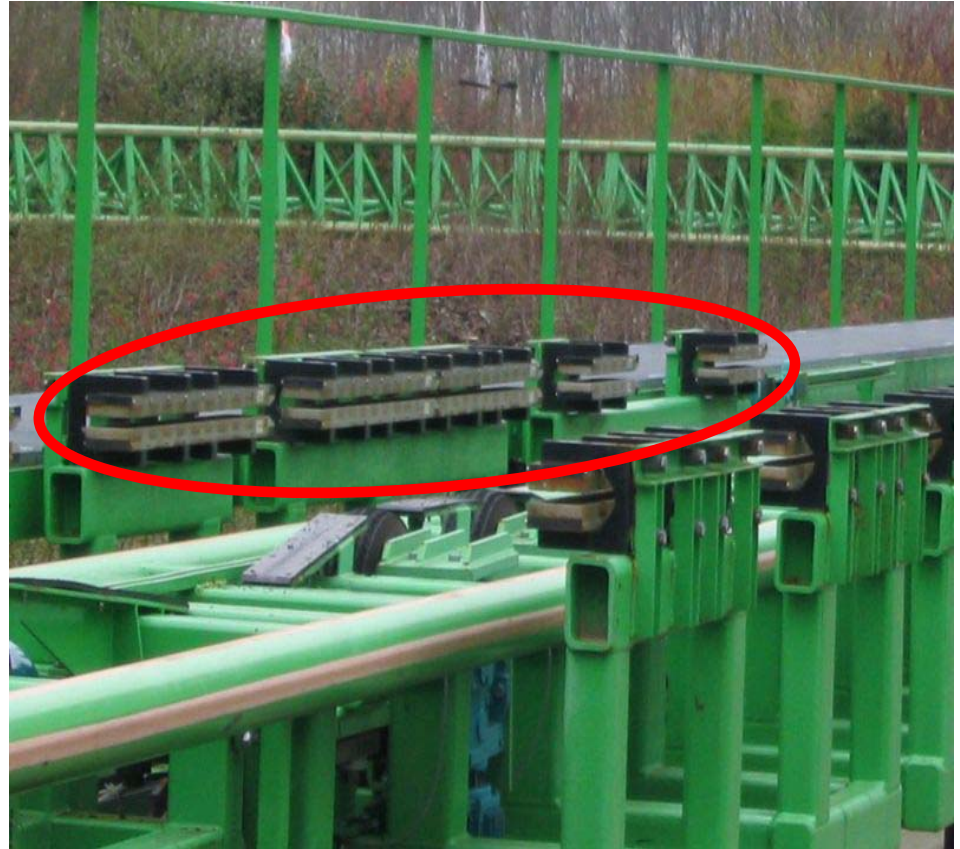
Goliath Roller Coaster at Walibi World in the Netherlands is stopped by eddy current brakes using permanent magnets instead of electromagnets
