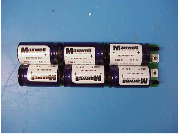
Fig. 2 D-cell module (6 cells, 350F, 2.5V each)
